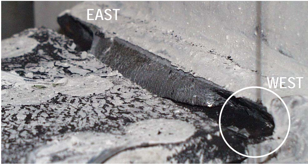
Figure 5.19 Photographs of fracture surfaces of MW-connections (Continued): (c) (Left) Top flange of Specimen MWI; and (d) (Below) Bottom flange of Specimen MWM
