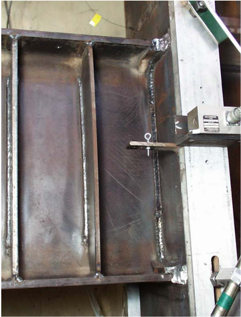
Figure 4.27 NA-Connection before testing: (a) (Left) Connection of Specimen NASL-RLP; and (b) (Above) Backing bar and reinforcement weld at link bottom flange (from Specimen NAM)
