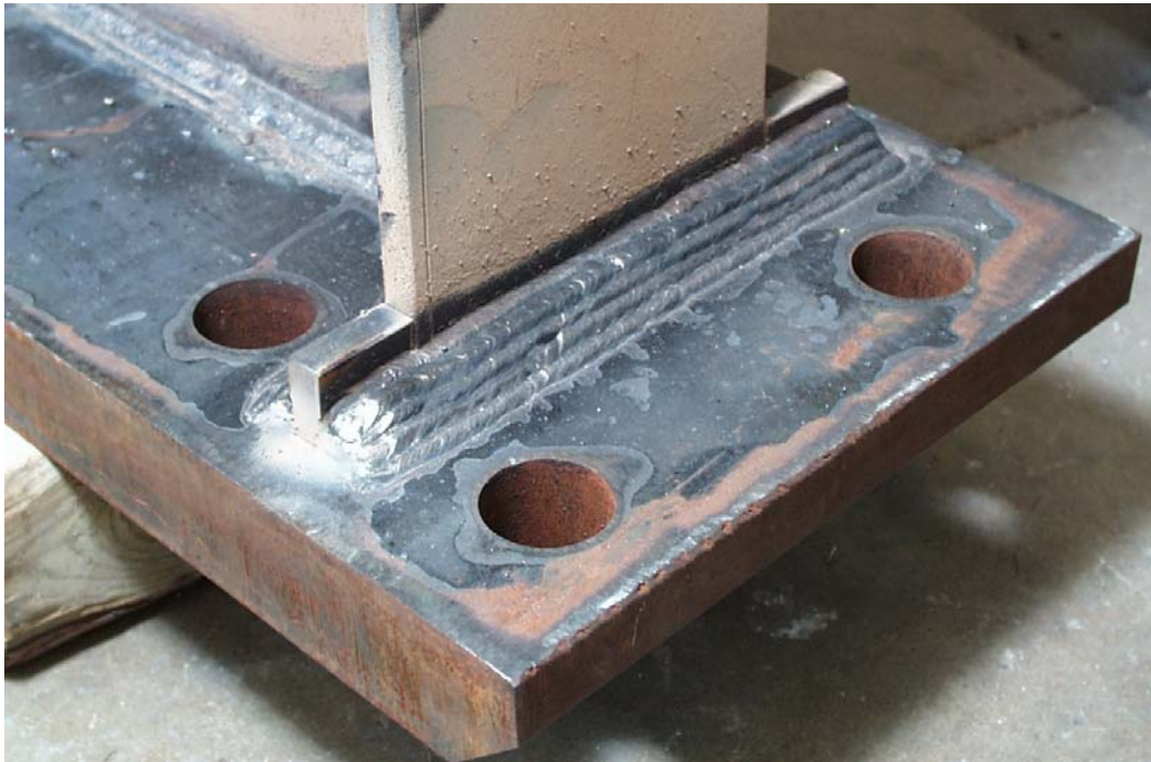
Figure A6 Typical end plate weld (Specimen PNI)
