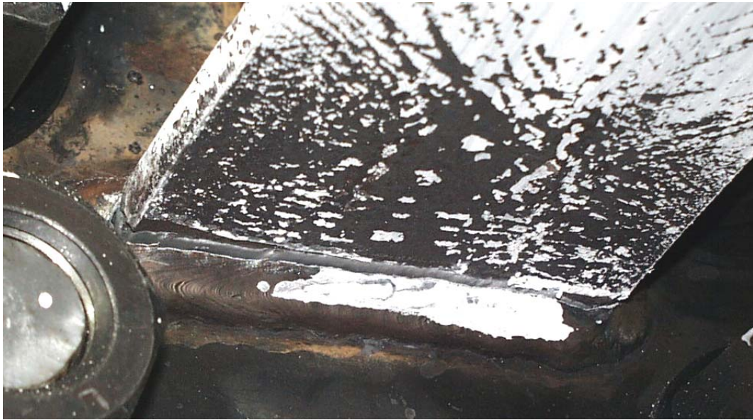
Figure A1 Fracture in Specimen 1A
