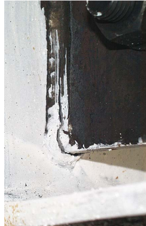
(b) Fracture in bottom edge of shear tab weld (0.06-1N)
