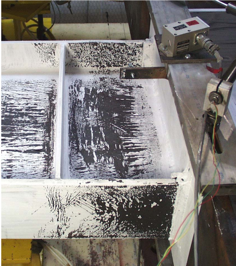
(a) Yielding in link near column face (0.04-2N)
