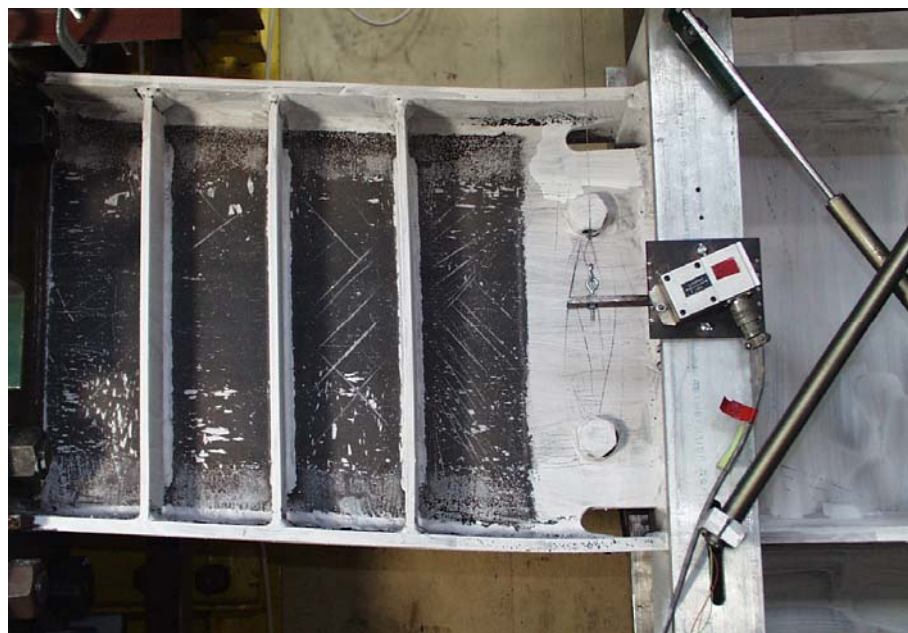
(b) Tested link and panel zone at \gamma = 0.06 rad
