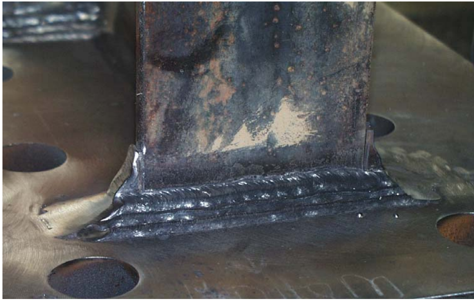
Figure A3 Fillet weld made for Specimen 1C
