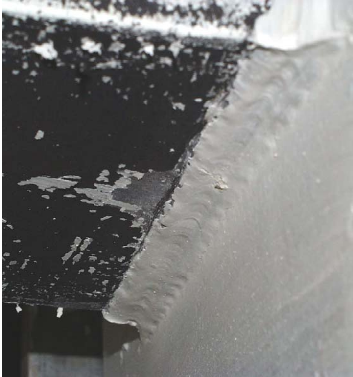
Figure 4.37 Photographs of Specimen NASL-RLP: (a) (Above) Fracture across link bottom flange (0.07-1N); and (b) (Right) Link top flange separated from column flange (0.09-1P)
