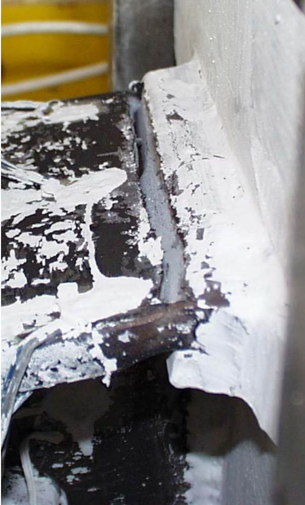
Figure 4.10 Photographs of Specimen MWS (Continued): (c) (Left) Link top flange separated from column face (0.07-2P); (d) (Above) Link after test
