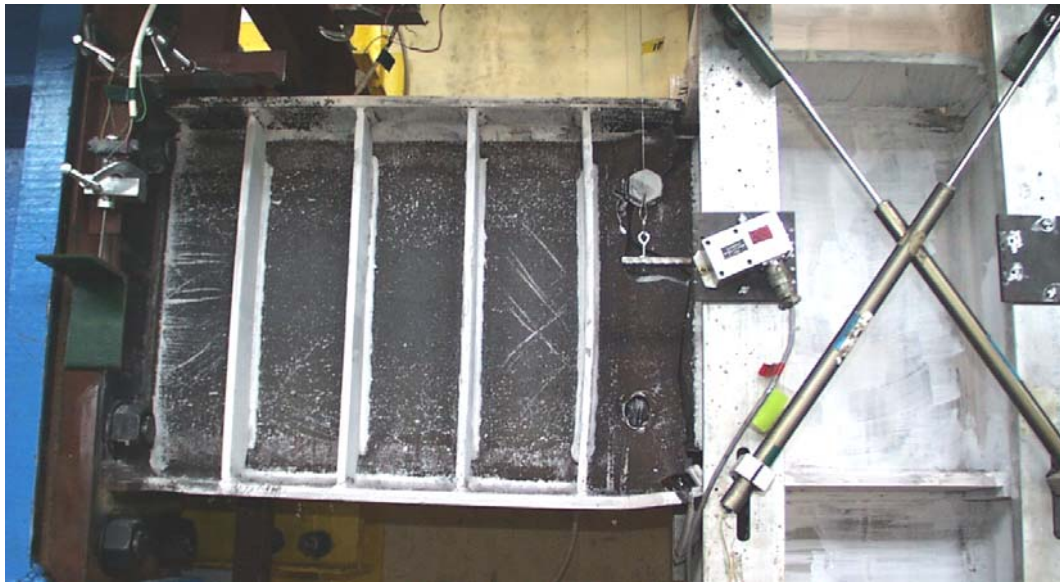
(b) Link and panel zone after test
