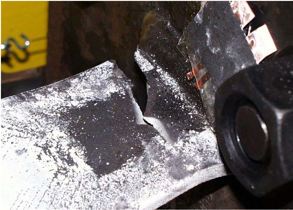
Figure A2 Fracture in Specimen 1B
