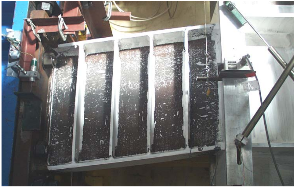
(a) Link deformation (0.13-1P)
