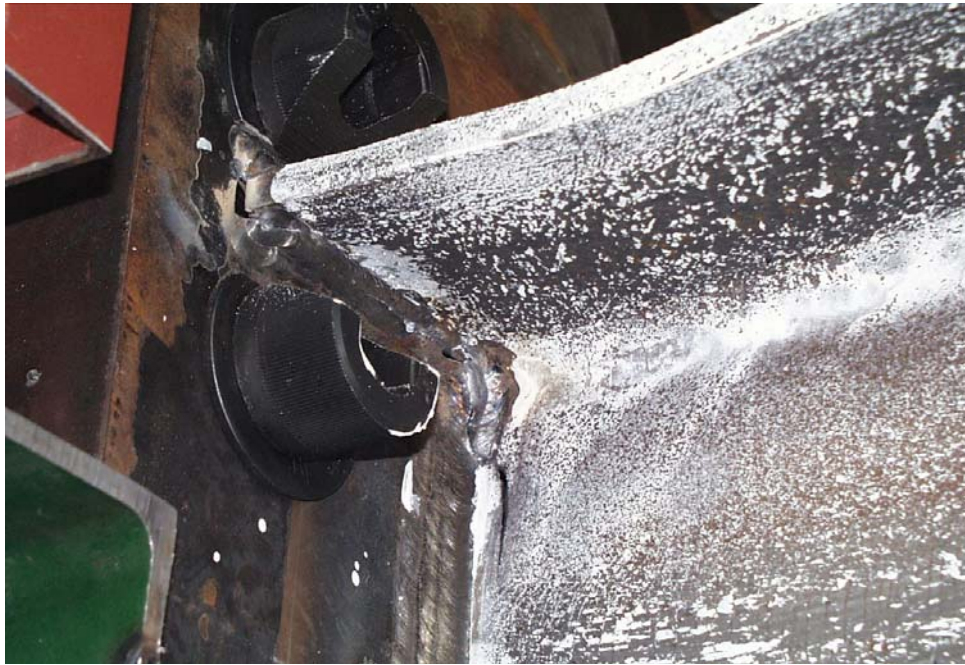
Figure A4 Fracture in Specimen 6A
