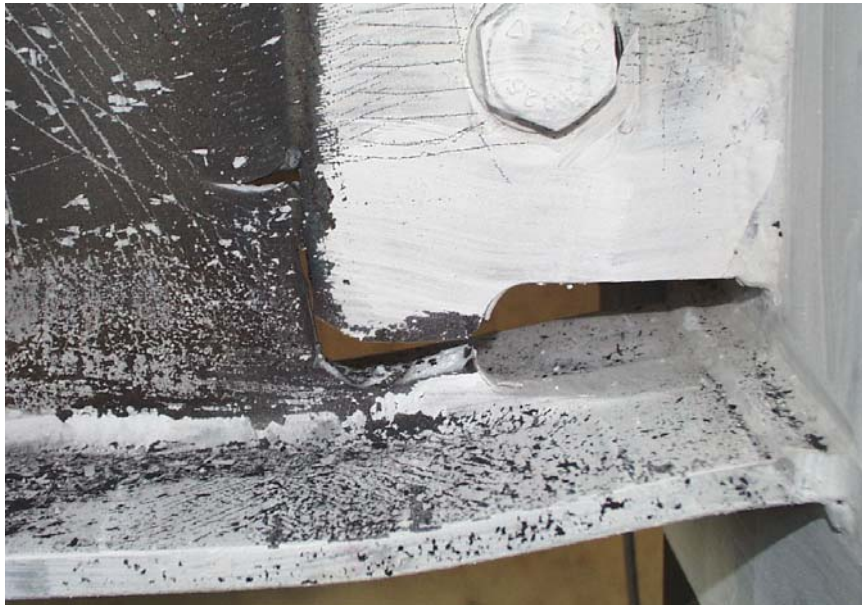
(b) Fracture in link web initiated at corner of shear tab (0.07-2P)
