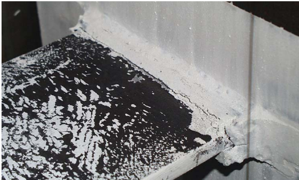
(b) Fracture in link top flange (after test)
