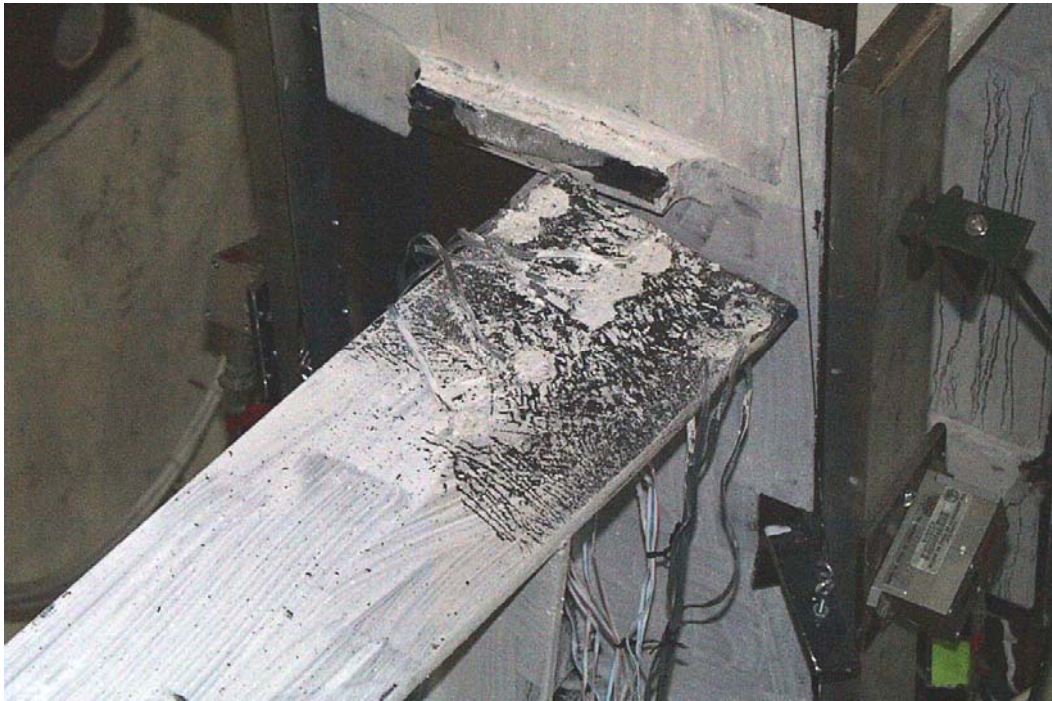
(c) Torsional deformation of link viewed from above the link (0.04-2N)
