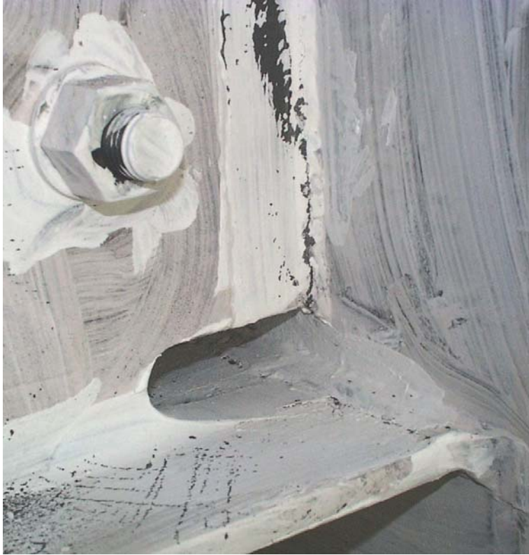
Figure 4.24 Photographs of Specimen FFS-RLP (Continued): (c) (Above) Fracture in bottom edge of shear tab weld (0.04-1N); and (d) (Right) Link-to-column connection after test
