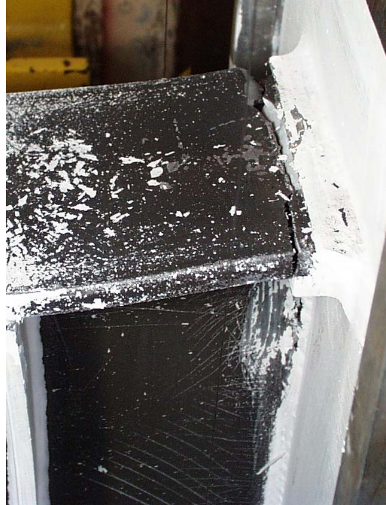
Figure 4.37 Photographs of Specimen NASL-RLP: (a) (Above) Fracture across link bottom flange (0.07-1N); and (b) (Right) Link top flange separated from column flange (0.09-1P)
