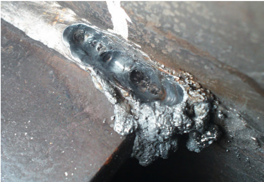
Figure E12 Discontinuity in link top flange of Specimen FFS-RLP
