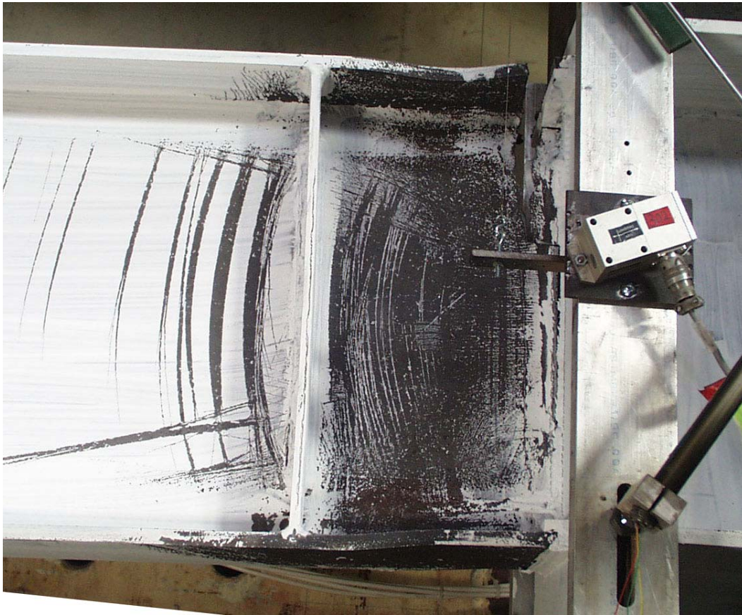
(c) Link-to-column connection after test
