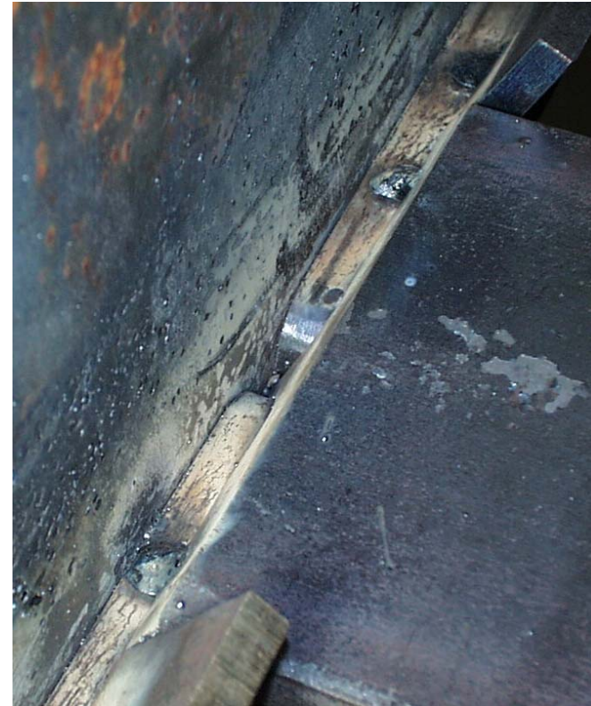
(b) Fabrication of Specimen NAI. Backing bar tack welded
