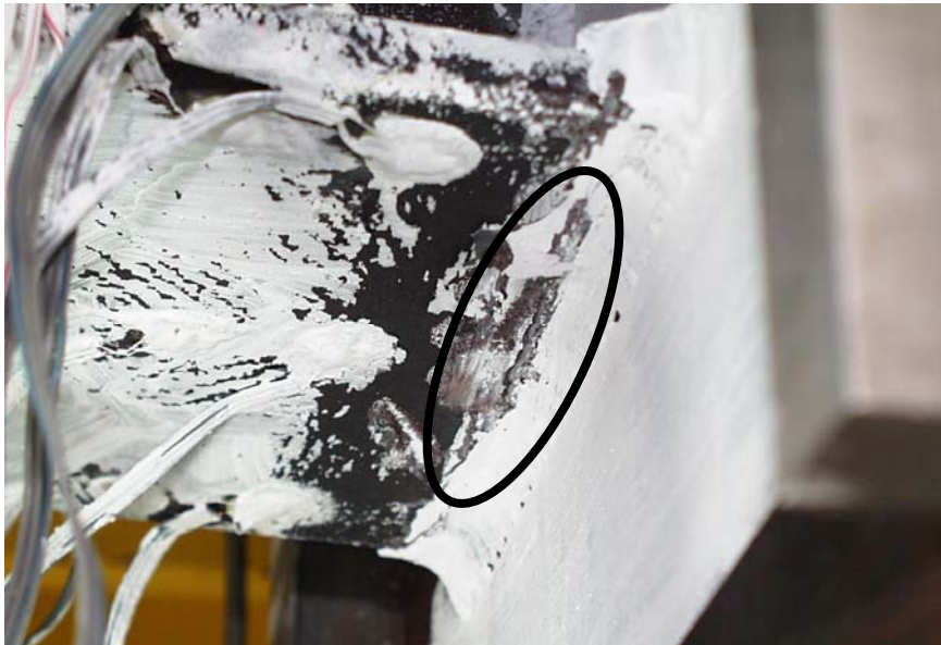
(a) Fracture in link bottom flange (0.06-2N)
