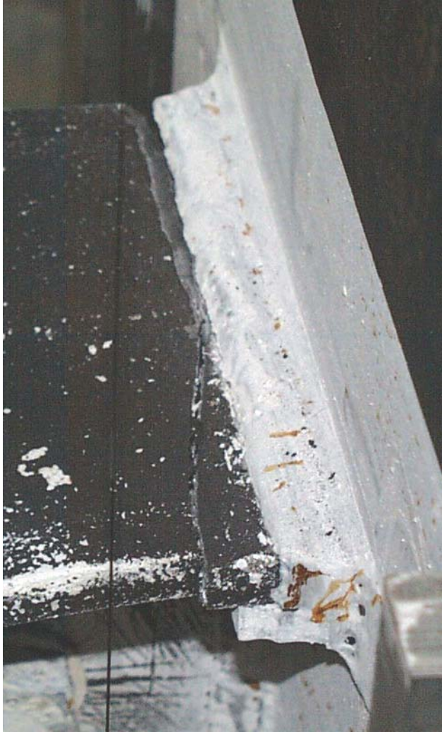
Figure 4.20 Photographs of Specimen FFI (Continued): (c) (Left) Link top flange separated from column flange (0.06-2P); (d) (Above) Link-to-column connection after test
