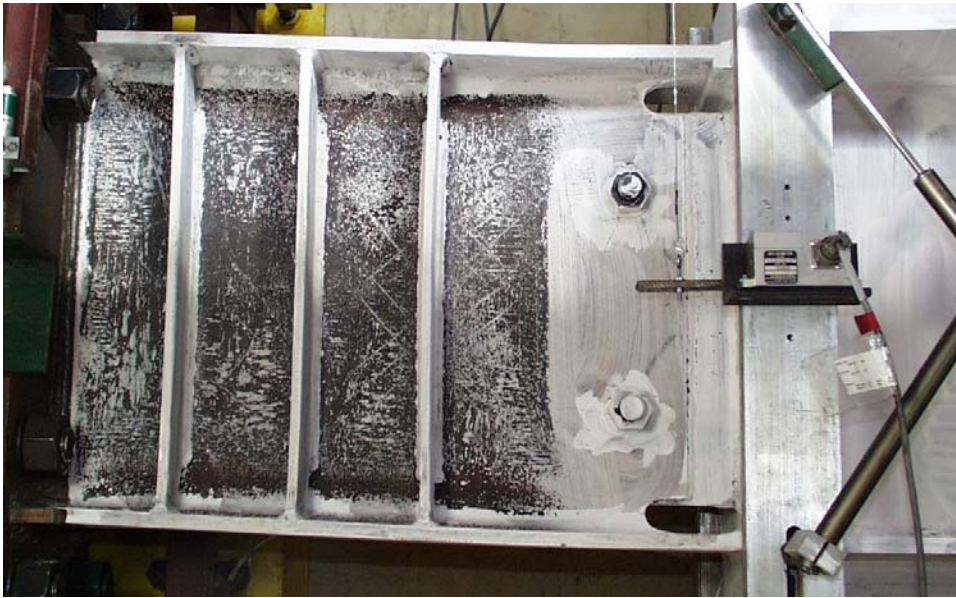
(a) Yielding in link web panels (0.03-2N)
